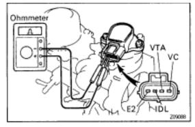
(d) Using an ohmmeter, measure the resistance between each terminal.
