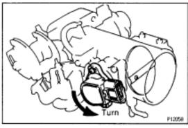
(e) Gradually turn the sensor clockwise until the ohmmeter deflects, and secure it with the 2 set screws.
