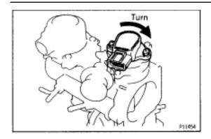
(d) Gradually turn the sensor clockwise until the ohmmeter deflects, and secure it with the 2 set screws.
