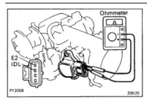
(d) Connect the tester probe of an ohmmeter to the terminals IDL and E2 of the sensor.
