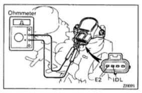
(c) Connect the tester probe of an ohmmeter to the terminals IDL and E2 of the sensor.
