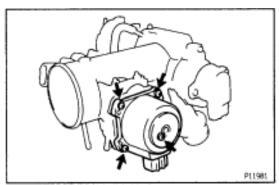
6. REINSTALL SUB-THROTTLE ACTUATOR
