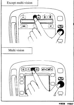
(3) All indication will illuminate as illustration, 4 times ON/OFF. And also buzzer will occur 4 times at the same time.
